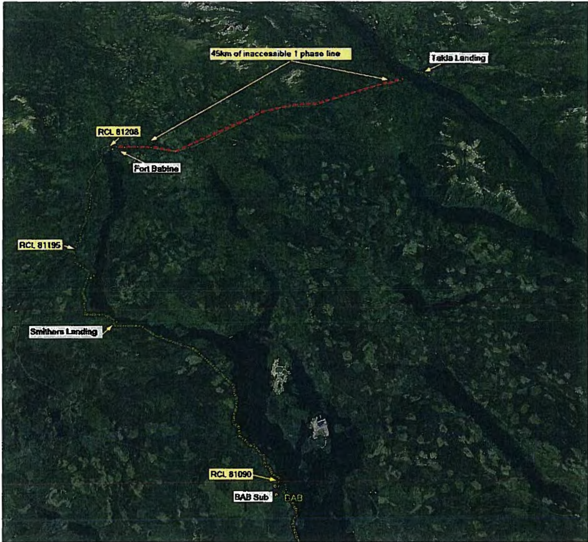
Figure 1: 45 km Electrical Supply Feeder to Takla Landing
