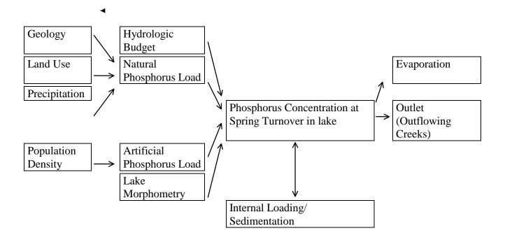
**FIGURE 2. Diagram of a Typical Nutrient Budget** (adapted from Dillon, and Rigler 1975). Total Nutrients into the lake minus the total nutrients out of the lake should equal the total phosphorus concentration in the lake at Spring turnover plus or minus the internal nutrient loading (if sediments are a source of the nutrient) or sedimentation rate (if sediments are a sink for nutrients).
