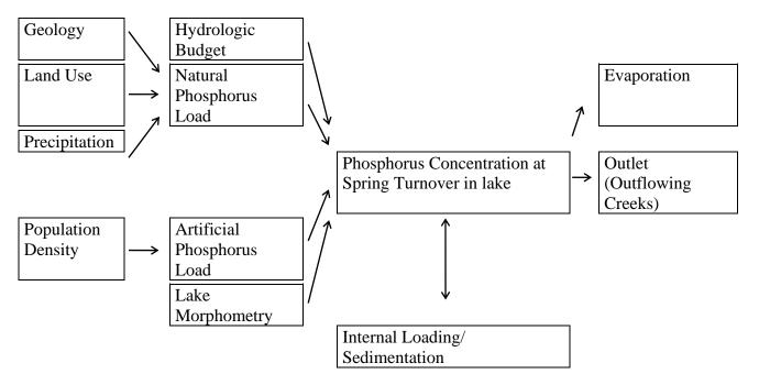
**Figure 2.** Diagram of a Typical Nutrient Budget (adapted by Rysavy and Sharpe, 1995, from Dillon and Rigler, 1975). Total Nutrients into the lake minus the total nutrients out of the lake plus or minus the internal nutrient loading (if sediments are a source of the nutrient) or sedimentation rate (if sediments are a sink for nutrients). should equal the total phosphorus concentration in the lake at spring turnover
