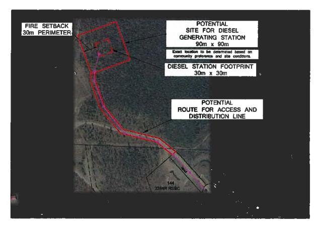
Figure 2 Proposed Permanent Diesel Generation Station Site
